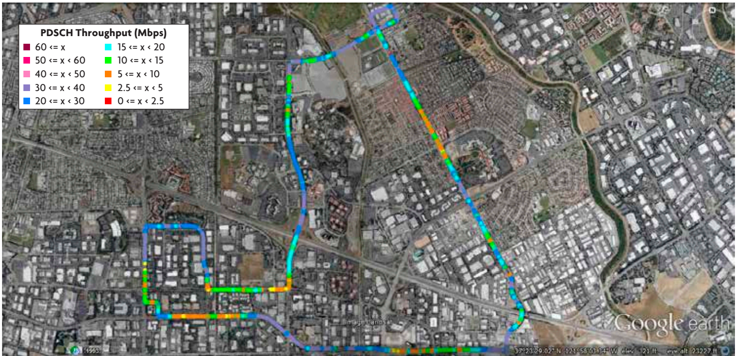
Figure 17. Physical Layer Throughput with TM 2 Only, July 19th, 0105 hours – Santa Clara Band 4 Network (geo plot)
