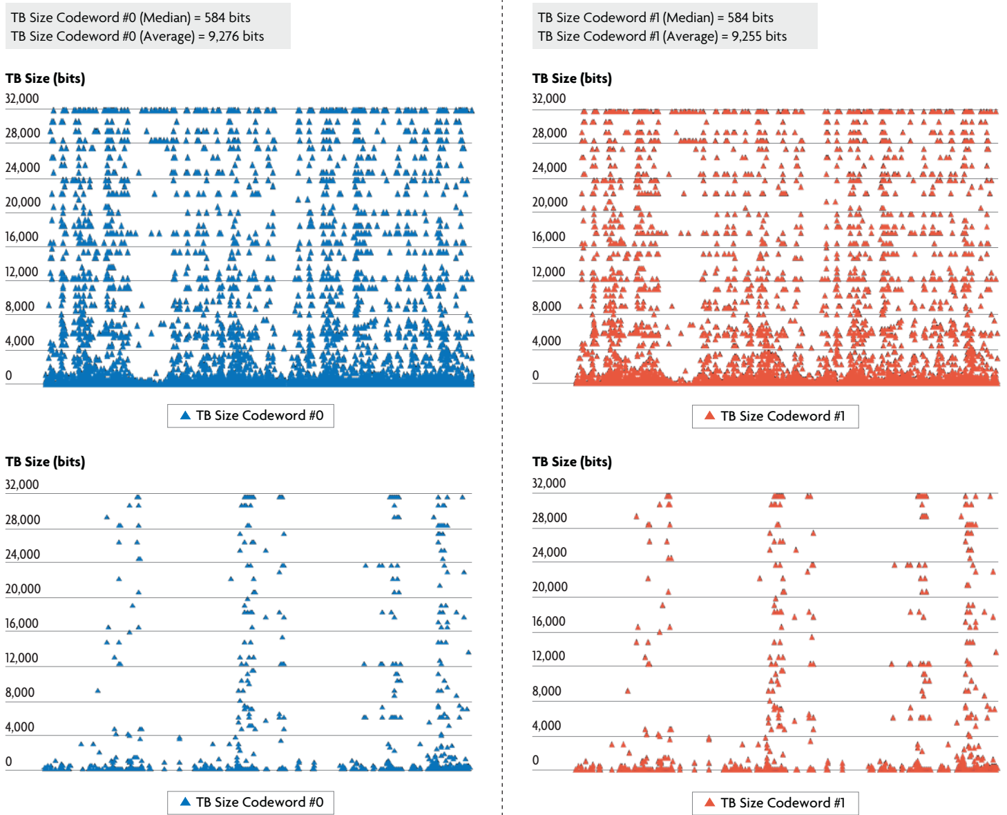
Figure 49. Transport Block Size Assignments with TM 3 Enabled with Web Browsing, Point 3 – Santa Clara, Band 4 Network
