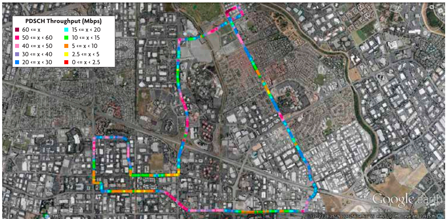
Figure 14. Physical Layer Throughput with TM 3 Enabled, July 18th, 0232 hours – Santa Clara Band 4 Network (geo plot)
