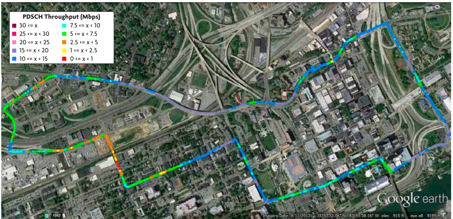
Figure 11. Physical Layer Throughput with TM 2 Only, July 19th, 0117 hours – Knoxville Band 5 Network (geo plot)
