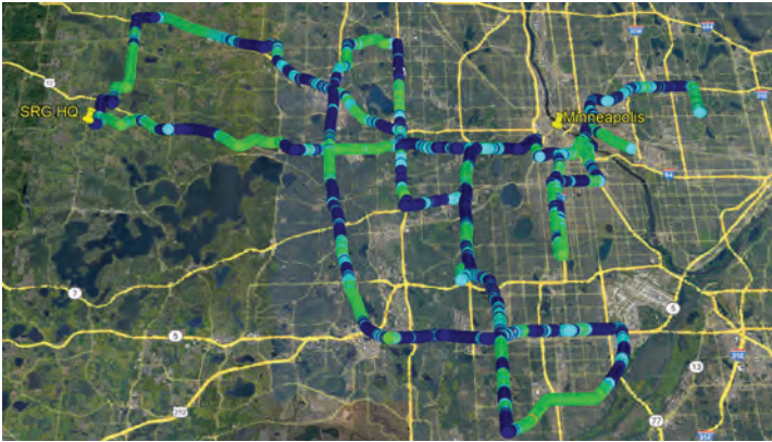
Figure 18. Low-band FDD 5G Coverage based on Signal Strength
