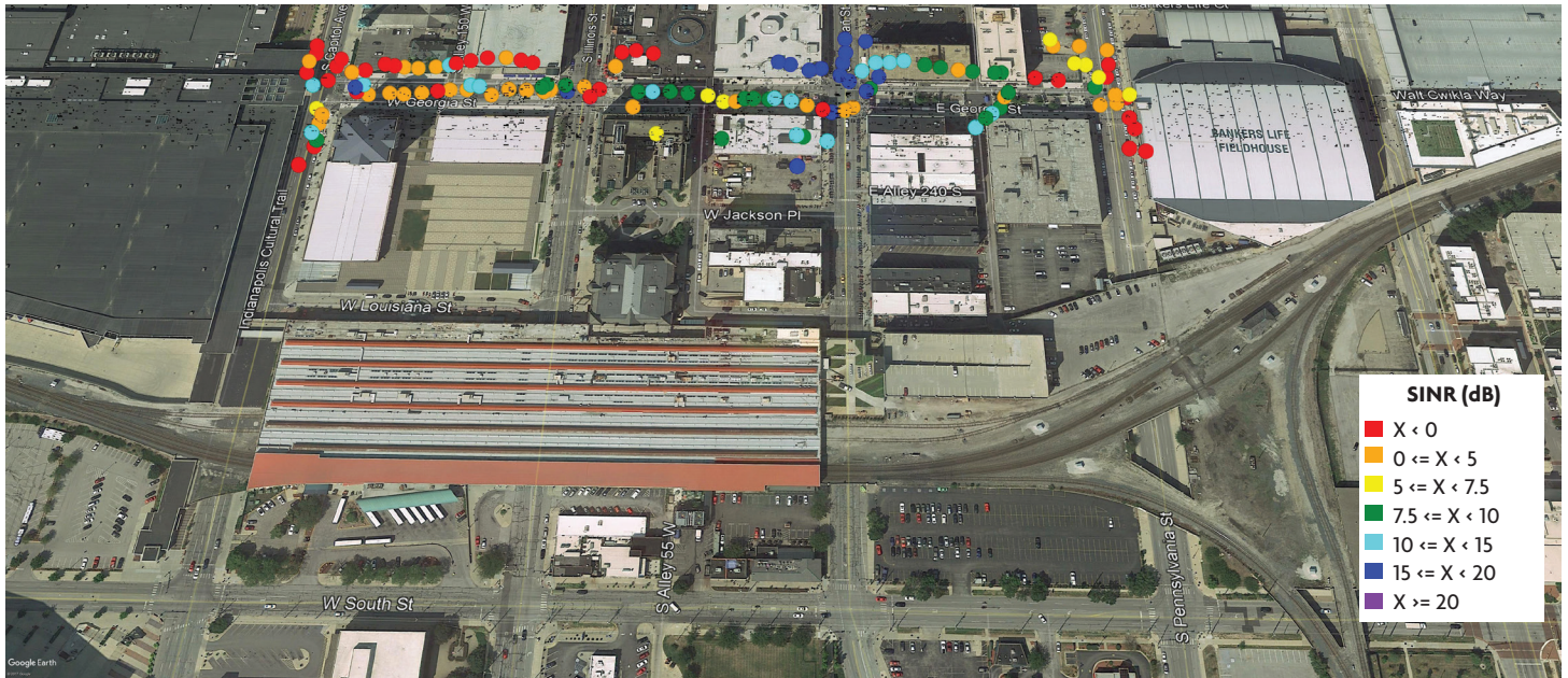
Figure 2. “Area 2” Binned SINR Values – minimal small cells (September)
