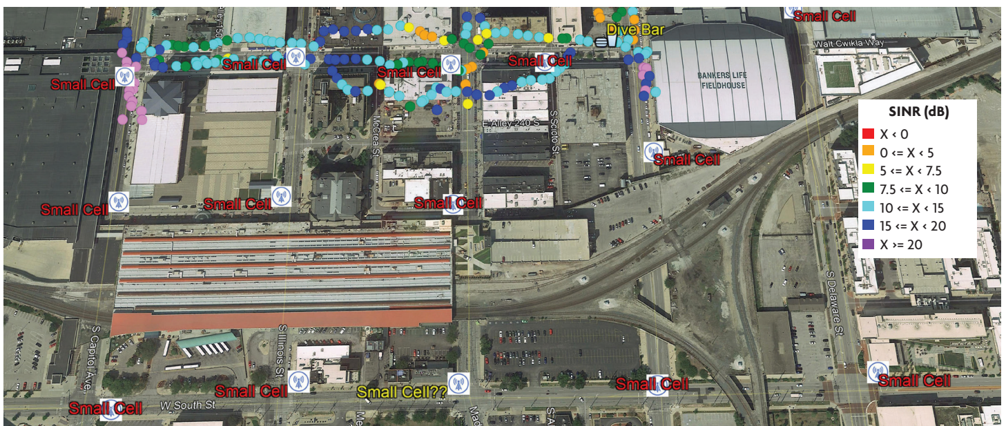
Figure 3. “Area 2” Binned SINR Values – with small cells (January)
